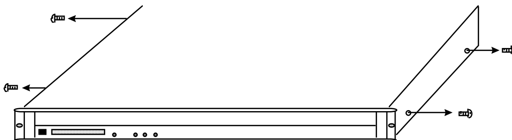
Figure 37 - Removing the Screws Securing the Cover
